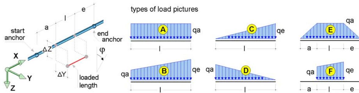
In the column "type" the load image type shown in the sketch and (separated by "/") the load direction of the line load is indicated.
