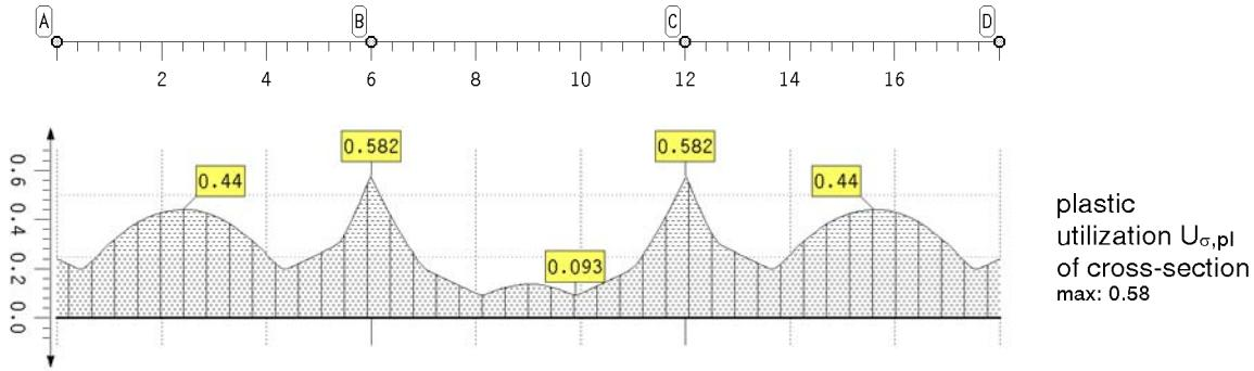
VERIFICATION 1: LOAD SPECTRUM 2: MCR: LOAD \* 1.61
