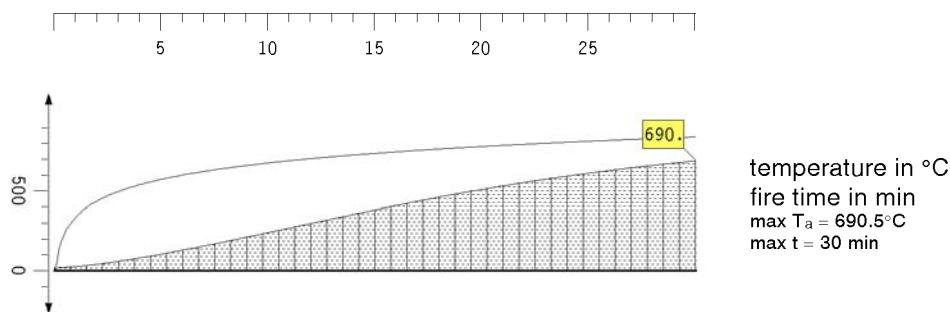
cross-section temperature acc. to  $t = 30$  min:  $T_a = 690.5$  °C
