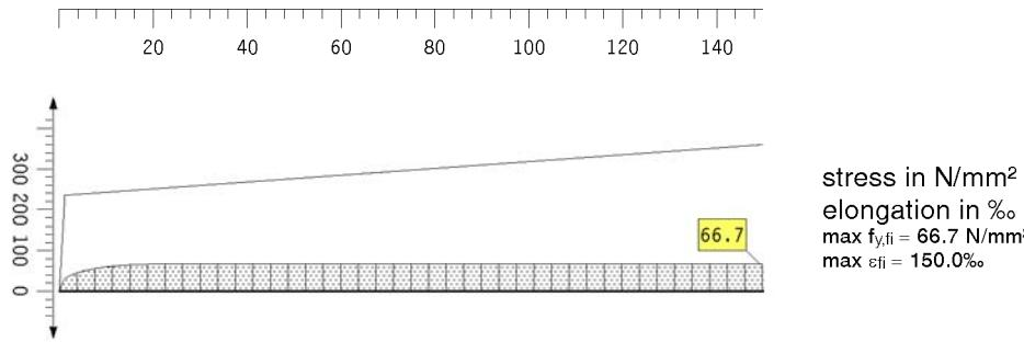
fire design with the simple design method s. EC 3-1-2, 4.2
