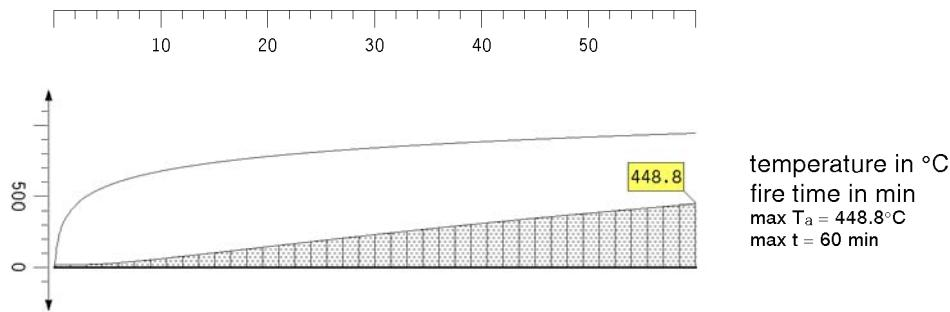
cross-section temperature acc. to  $t = 60.0 \text{ min}$ :  $T_a = 448.8^\circ\text{C}$
