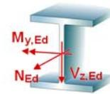
local stresses especially of the beam and of welds are not considered !
