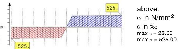
stress-strain line of concrete: EC 2-1-1, 3.1.5 (realistic)
