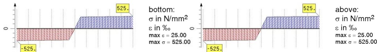
stress-strain line of concrete: EC 2-1-1, 3.1.5 (realistic)
