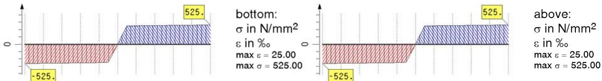
stress-strain line of concrete: EC 2-1-1, 3.1.7 (parabola-rectangle diagram)
