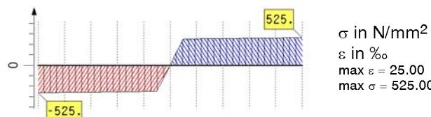
stress-strain line of concrete: EC 2-1-1, 3.1.7 (parabola-rectangle diagram)
