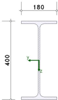
elastic cross-sectional check for  $M_{Ed} = -30.13 \text{ kNm}$ ,  $V_{Ed} = 163.10 \text{ kN}$
