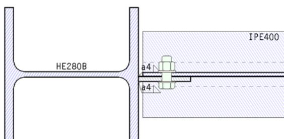
beam connection with fin plate, connected to the flange of the main girder
