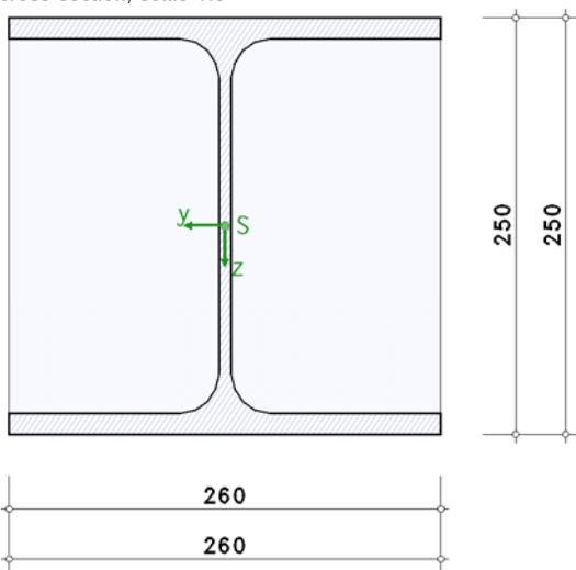
**column cross section with clamping depth  $f = 60.0 \text{ cm}$**
